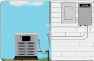
An automatic standby generator works by monitoring utility voltage 24/7. When your electricity is interrupted, the generator detects the problem and goes to work. The automatic transfer switch safely disconnects the utility line and transfers to generator power. Power is simultaneously restored within seconds. Once the utility is restored, the generator returns to standby mode.
